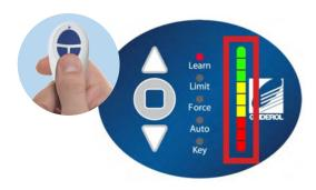
Press and hold the desired button for operation on the handset. Hold down until every light in the status bar on the powerhead (as shown above) is lit up.
