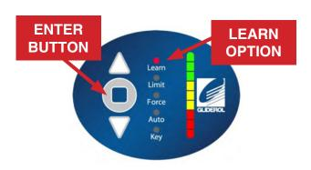
Use the arrow (Up & Down) buttons to select the 'Learn' option and press 'Enter' to confim selection. The unit will beep three times to confirm the unit is in Learn mode.
