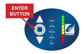
Press and hold the 'Enter' button (shown above) for 2 seconds to access the operator menu. The unit will beep twice to confirm this has been selected.
