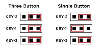
The factory setting on your opener is three button operation. to enable single button operation, reconfigure the key shunts as per the above diagram.
