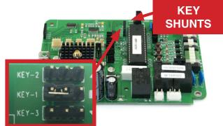
Locate the three key shunts on the main control board (adjacent to the receiver board). These are labelled KEY-2, KEY-1 & KEY-3 and correspond to the buttons on your remote.
