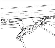
Once installed, prior to configurating your opener attach the stopping mechanism as shown below with your door in the fully opened position (refer below). This will avoid the carriage overrunning during limit and force settings.
