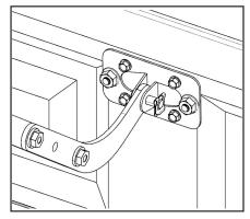
Use the below examples as a guide when positioning you door hinge and J-arm. Ensure J-arm does not touch bracing etc during normal operation. Attach manual release cord to complete installation.
