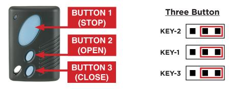
Relocate the jumpers to the last two pins (on the right hand side) adjacent to each key label as per the above diagram. Jumpers are the small, black sleeves that slide over the key shunts and one is shown in the KEY-1 position in Step 2.
