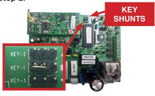
Locate the three key shunts on the main control board (adjacent to the receiver board). These are labelled KEY-2, KEY-1 & KEY-3 and correspond to the buttons on your remote.
