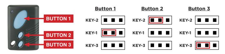
Note: To operate multiple doors (up to 3) from one remote, simply place a second jumper adjacent to the desired key label
