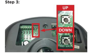
Press and hold the 'UP ADJ' button until the door travels to the desired open position. Press 'Limit' once to save this position in the units memory. Unit will beep twice to confirm. Repeating this process, press and hold the 'DN ADJ' button until the door reaches the desired close position. Press the 'Learn' button to save. Your travel limit setup is now complete!
