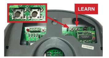
Press and hold the 'Learn' button for three seconds. The unit will beep three times to confirm the unit is in learn mode.
