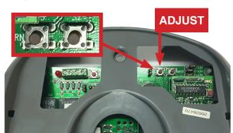
Press and hold the 'ADJ' button (located next to the 'Learn' button) until the door travels to the desired open position. Press 'Learn' once to save this position in the units memory. Unit will beep twice to confirm. Repeating this process, press and hold the 'ADJ' button until the door reaches the desired close position. Press the 'Learn' button to save. Your travel limit setup is now complete!
