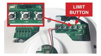
Press the 'Limit' button once. The unit will beep three times to confirm the unit is in limit setting mode mode.
