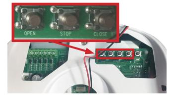
Set the top/open door limit by using the 'Open' and 'Close' buttons to raise the door to it's open position. Press 'Stop' to confirm limit. Set the bottom/close door limit by using the same 'Open' and 'Close' buttons to lower the door to it's closed position. Press 'Stop' to confirm limit.
