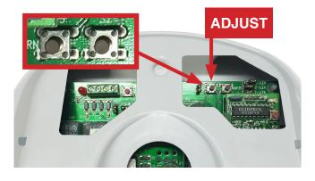
Press and hold the 'ADJ' button (located next to the 'Learn' button) until the door travels to the desired open position. Press 'Learn' once to save this position in the units memory. Unit will beep twice to confirm. Repeating this process, press and hold the 'ADJ' button until the door reaches the desired close position. Press the 'Learn' button to save.
