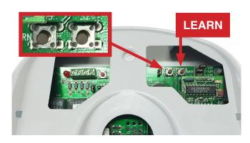
Press and hold the 'Learn' button for three seconds. The unit will beep three times to confirm the unit is in learn mode.
