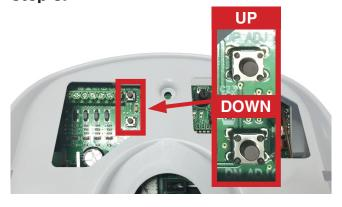
Press and hold the 'UP ADJ' button until the door travels to the desired open position. Press 'Limit' once to save this position in the units memory. Unit will beep twice to confirm. Repeating this process, press and hold the 'DN ADJ' button until the door reaches the desired close position. Press the 'Learn' button to save.
