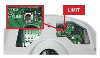
Press and hold the 'Limit' button for three seconds. The unit will beep three times to confirm the unit is in limit setting mode.
