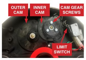
Loosen the three cam gear screws. To set the close position, manually lower the door to the desired position whilst observing the direction of rotation of the inner most cam. Rotate the inner cam in the direction observed until it activates the inner limit switch.
