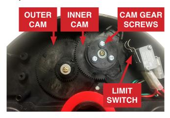
To set the open position, manually raise the door to the desired position (ensuring the botom bar is short of contacting the guide stop) whilst observing the direction of rotation of the outer cam. Rotate the outer cam in the direction observed until it activates the inner limit switch.
