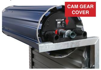
Set the door to manual operation (refer Glidermatic GRD Manual Operation Guide for details) and carefully remove the cam gear cover to gain access to the internal cams .
