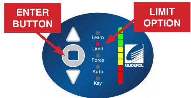
Use the arrow (Up & Down) buttons to select the 'Limit' option and press 'Enter' to confirm selection.
