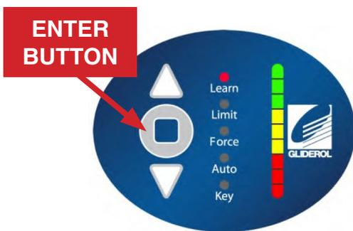
Press and hold the 'Enter' button (shown above) for 2 seconds to access the operator menu. The unit will beep twice to confirm this has been selected.
