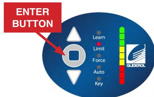
Upon reaching the floor, the unit will beep 3 times to confirm floor level has been reached. You can then set the top/open door limit by using the arrow (Up & Down) buttons on the operator (or the buttons on your Gliderol Handset) to raise the door curtain to it's open position. Press 'Enter' to confirm limit.
