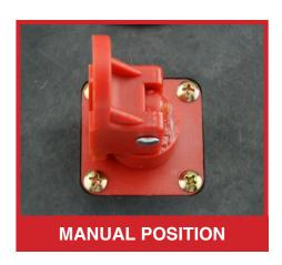
To put the door into manual operation mode, flip the red manual release lever (located at the end of your roller door curtain) 90 degrees so that it is pointing toward you. Your door can now be manually operated.
