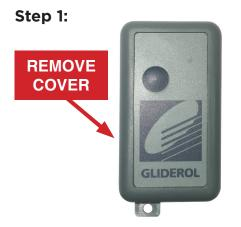
Remove the cover from the handset to expose the handset circuit board.
