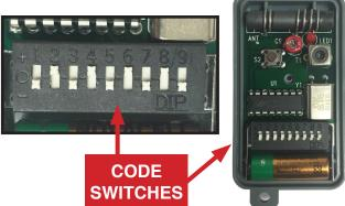
Push the numbered switches 'up' or 'down' to reflect the same code shown inside your existing control box.
