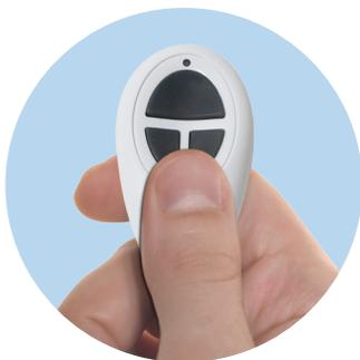
Press the button on the handset that you would like to operate the door. The unit will beep once to confirm successful coding (two beeps indicates the handset has already been programmed). Wait approx 3 seconds for the unit to exit setup mode.
