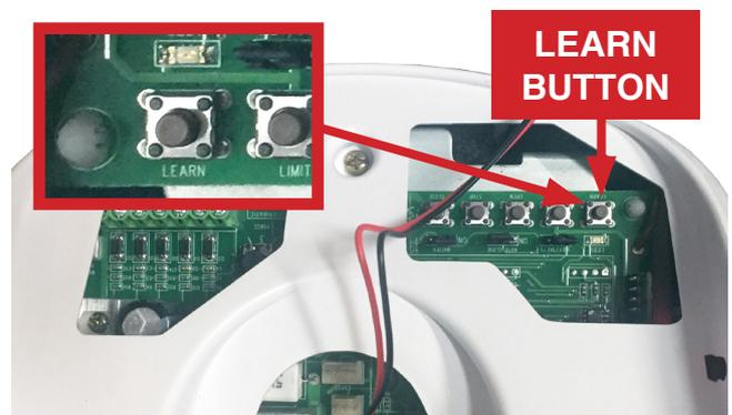
Press the 'Learn' button once. A red light will illuminate and the unit will beep three times to confirm the unit is in learn mode.
