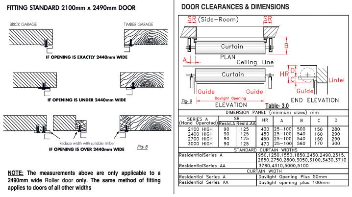
Important Note: The fixings to the bracket supplied in the parts bag is specifically for timber fix only. If the bracket is to be fixed to brick or other members the installer should find the right fixing by referring to table 2.0 for maximum pull out strength requirements. Gliderol warranty voids and no responsibility accepted by the manufacturer if the door is not installed as per the installation instructions.
